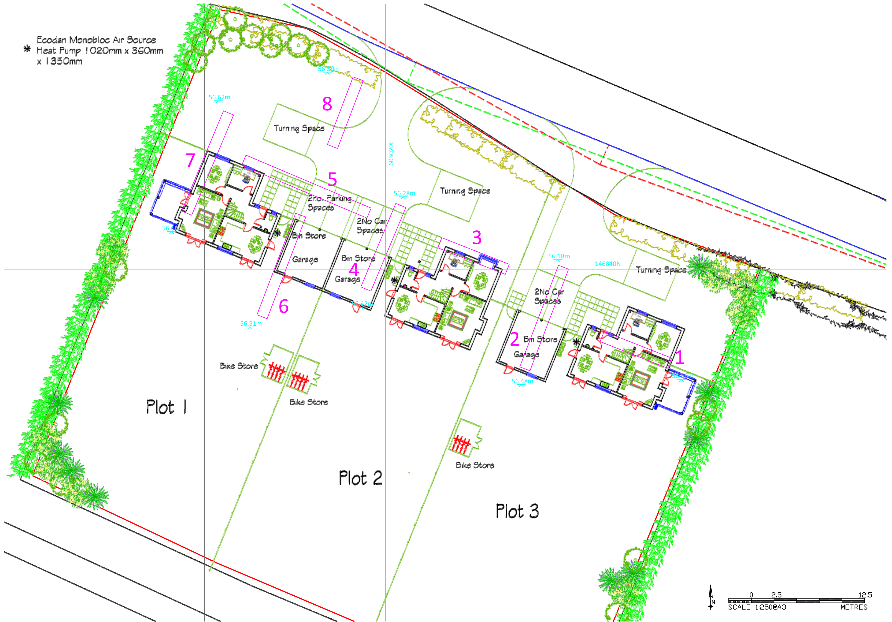
Figure 4: Trench location in relation to development
